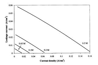
Fig. 6 Methanol crossover for different methanol bulk concentrations
