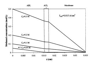
Fig. 5 Concentrations profiles for different methanol bulk concentrations
