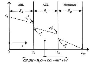
Fig. 3 Schematic of the DMFC layers considered in the model
