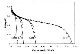
Fig. 4 Model predictions for different methanol concentrations
